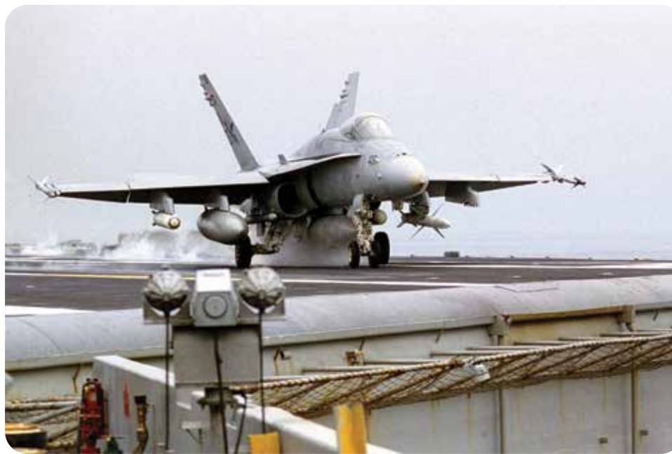
A US Navy F/A-18C Hornet launches from USS Nimitz carrying CBU-100 cluster bombs.
