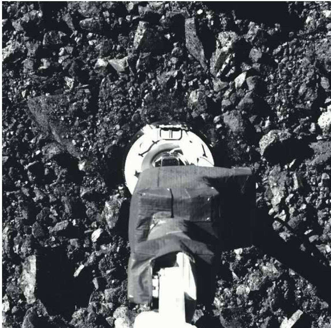
The Origins, Spectral Interpretation, Resource Identification, Security, Regolith Explorer (OSIRIS-REx) spacecraft unfurled its robotic arm in October 2020, and in a first for the agency, briefly touched an asteroid to collect dust and pebbles from the surface for delivery to Earth in 2023. Photo: NASA/Goddard/University of Arizona
